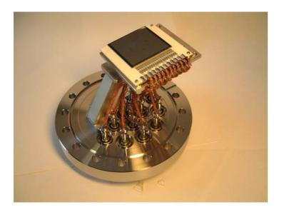
active area: 40 x 40 mm<sup>2</sup>, thickness: 1 mm, UHV compatible
