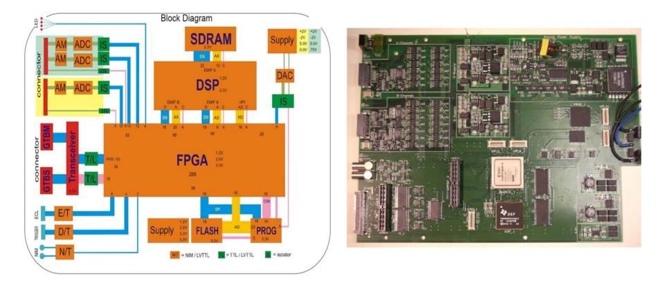
Up to 15 detectors could be readout by SIDEREMs and single SAM module All modules and SAM are connected by GTB interface (data rate up to 5 Mb/s)
