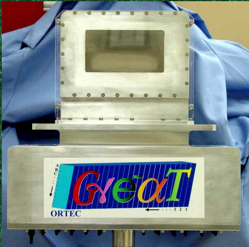
GREAT planar germanium detector for focal plane spectroscopy of gammas and betas
