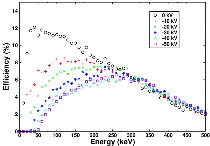
**Figure 3.** Effect of HV barrier on electron transmission for different barrier voltages. At higher energies the curves are identical. The amount of lower energy electrons that reach the detector reduces with increasing barrier voltage. The simulations were performed with 1000 A current through the coils and no helium present in the target chamber.
