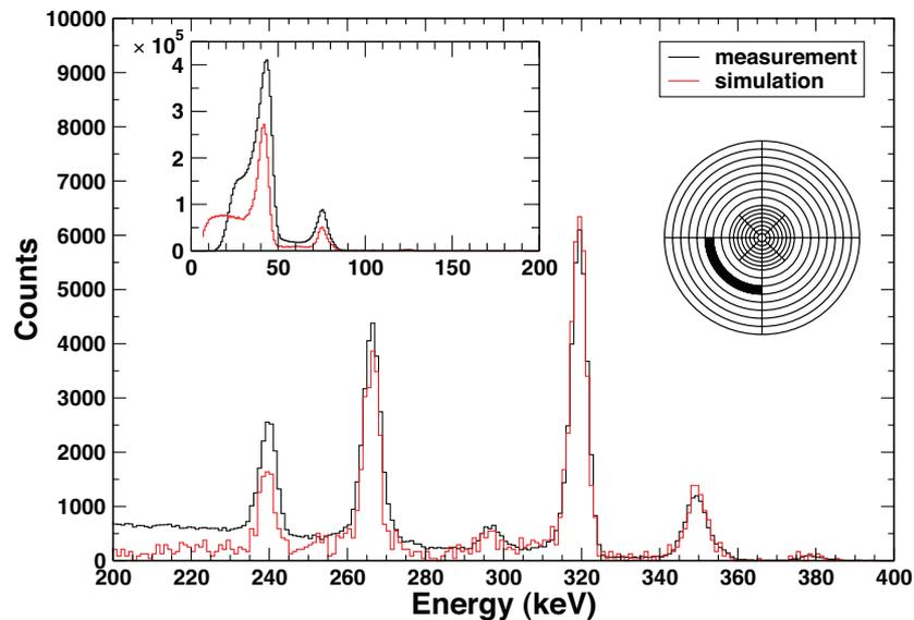
**Figure 4.** Comparison between measured (black) and simulated (red)  $^{133}\text{Ba}$  spectra from the same detector pixel, shown in the detector diagram on the right. The inset shows the lower energy peaks.
