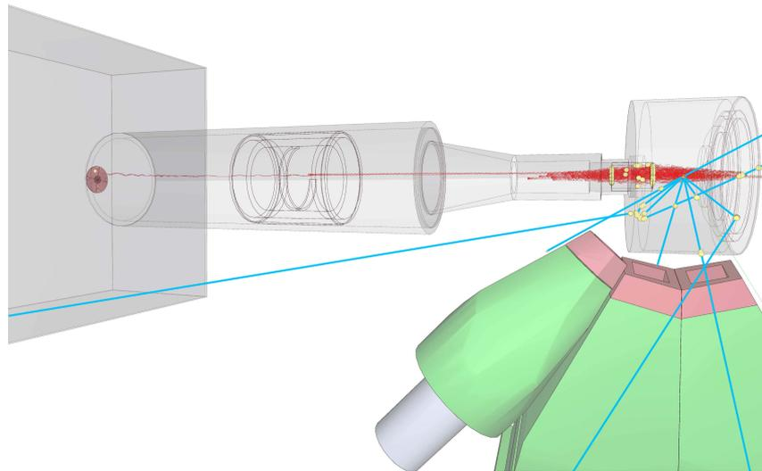
**Figure 5.** Example of simulated events visualised in Geant4. Electrons are presented with red lines and  $\gamma$  rays with blue. Some of the electrons reach the detector while the rest either interact with the surrounding material or are reflected by the HV barrier.
