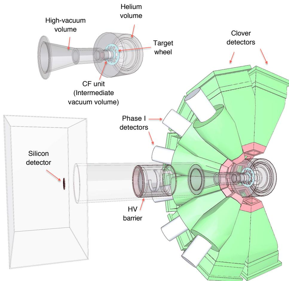
**Figure 1.** Schematic representation of the simulated volume. One half of JUROGAM II is drawn for graphical reasons. The main parts of the geometry are indicated on the figure. A detail of the target region is shown on the top left part of the figure.
