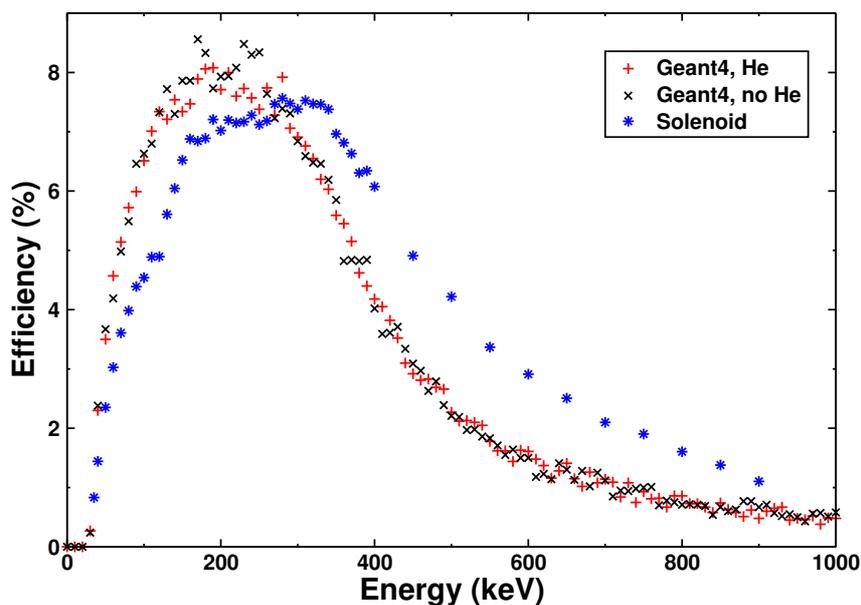
**Figure 2.** Simulated transmission and detection efficiencies obtained with Geant4 with and without helium at the target chamber compared with an efficiency plot obtained with SOLENOID without using helium. The simulations were produced with 1000 A current through the coils and -30 kV on the HV barrier.
