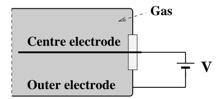
Virtually any gas can be used for the chamber, air being the most common. Denser gases may be used to increase the ionisation density. Charged particles ionise the gas into electrons and positively charged molecules. An electric field prevents electrons and ions of the absorber recombining and they drift in opposite directions producing an ion current, which is measured.
