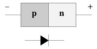
When p- and n-type materials are brought into contact, charge migrates and creates a region free from charge carriers around the interface. This depletion layer forms the active volume of a semiconductor radiation detector. The depletion layer has a charge carrier density of  $10^2\ cm^{-3}$  compared with  $10^{10}\ cm^{-3}$  outside the layer.
