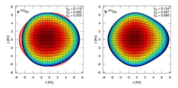
Figure 4. Graphical representation of the shapes of (a)  $^{220}$ Rn and (b)  $^{224}$ Ra. Fig. (a) depicts vibrational motion about symmetry between the surface shown and the red outline, while (b) depicts static deformation in the intrinsic frame. Theoretical values of  $\beta_4$  are taken from ref. 10. The colour scale, blue to red, represents the y-value of the surface.
