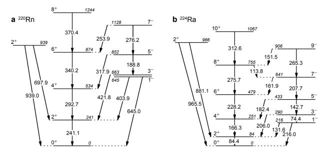
Figure 2: Partial level-schemes for  $^{220}$ Rn (a) and  $^{224}$ Ra (b) showing the excited states of interest for this work. Arrows indicate known  $\gamma$ -ray transitions. All energies are in keV and spins in units of  $\hbar$ . Note that the level at 939 keV in  $^{220}$ Rn is observed for the first time in this work.
