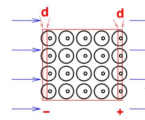
Similarly on the other side. Electrons have been sucked out of this strip, and at the surface of the material they cannot be replenished, therefore we build up a net positive charge.
