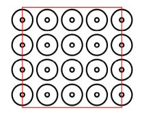
As *all* negative charges move against  $\vec{E}$  and *all* positive charges move with  $\vec{E}$ , we build up surface charges: Consider a small unit volume inside the insulator.
