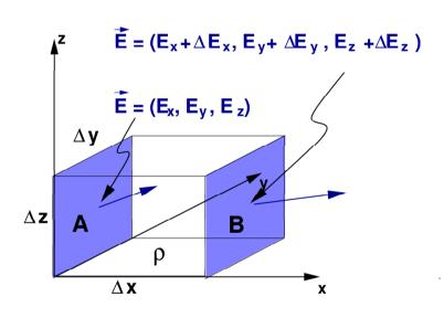
$$\Phi = \left[ \frac{\partial E_x}{\partial x} + \frac{\partial E_y}{\partial y} + \frac{\partial E_z}{\partial z} \right] \Delta x \Delta y \Delta z$$
