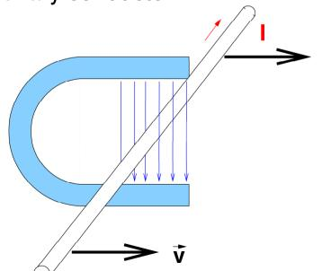
A) moving conductor, stationary magnet The conductor cuts through the  $\vec{B}$ , thus the charges moving with the conductor experience a Lorentz force and a current flows. In the picture the current flows into the page.
