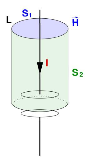
Consider a straight wire that charges a capacitor. We calculate the magnetic field strength  $\vec{H}$  via the surface  $S_1$  shown in the figure. Clearly  $\vec{H} \neq 0$ , and more precisely
