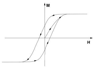
The magnetic moments of the material are so large that they align each other into magnetic domains. The magnetization of each domain is completely saturated.
