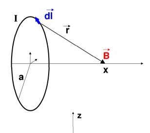
Here we shall consider a circular loop of radius a in the y-z plane. The loop carries a current I moving clockwise looking in positive x-direction and we want to evaluate the magnetic field on a point  $\vec{r}_0 = (x, 0, 0)$  on the x-axis.
