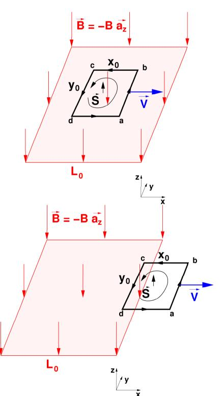
As the rectangle is fully in the field, the contributions  $a \to b$  and  $d \to c$  are equal and opposite: no current flows.
