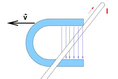
B) stationary conductor, moving magnet
