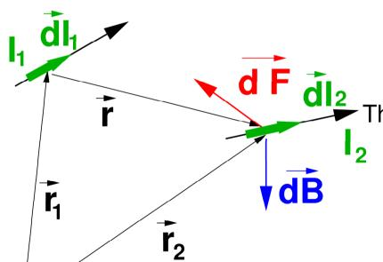
$$d\vec{B} = \frac{\mu_0}{4\pi} \frac{I_1 \, d\vec{l}_1 \times (\vec{r}_2 - \vec{r}_1)}{|\vec{r}_2 - \vec{r}_1|^3}$$
