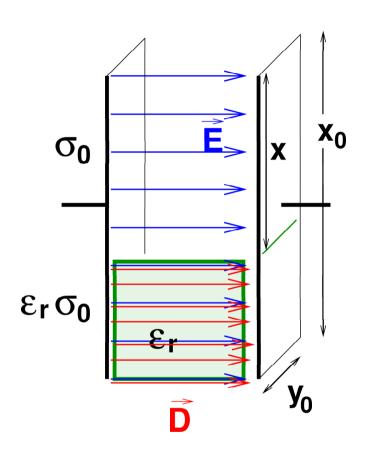
Now we must deduce the exact field configuration in the capacitor if it is partially filled with a dielectric.
