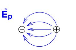
The electric field inside the dielectric is reduced because field lines can now start and end on the induced surface polarization charges. If you look more closely you will note that the electric field from each dipole is oriented opposite the external field. The net field is the sum of both, and we get a reduction of  $\vec{E}$  .
