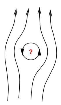
Can an electrostatic field contain closed loops? Then we could evaluate the path integral  $\oint \vec{E} \, dl$  around such a loop an get a numerical value different from zero, i.e. we could put a charge onto the loop and it would continually "ride round". This is in contradiction to the assumption of electrostatics. We shall prove this more formally:
