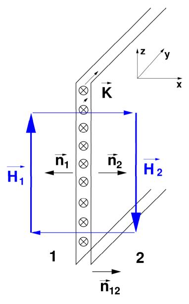
First we calculate the magnetic field created by that current sheet. We call the surface current density  $\vec{K}$ . From Ampere's law we can calculate  $\vec{H}$  on either side:
