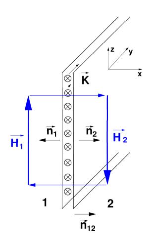
Now we split the magnetic field  $\vec{H}$  up into a part generated by the current sheet  $\vec{H}_K$  and one generated by all other currents  $\vec{H}_O$ :
