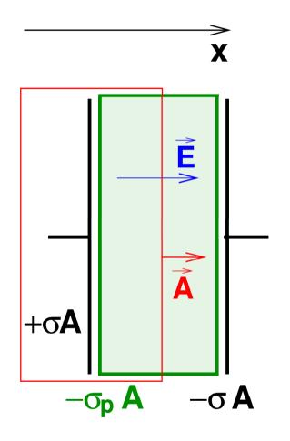
Now the slab of dielectric enters the space between the plates leaving a tiny gap on either side. We keep the potential difference fixed at  $\Delta V$ . Polarization charges appear and in the vast majority of the volume the electric field is reduced:
