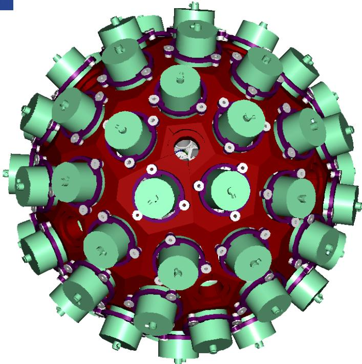
The innovative use of detectors (**pulse shape analysis,  $\gamma$ -ray tracking, digital DAQ**) will result in high efficiency (~40%) and excellent energy resolution, making AGATA the ideal instrument for spectroscopic studies of weak channels.
