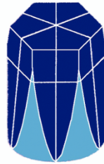
MINIBALL triple-clusters with 6 and 12 fold segmentation
