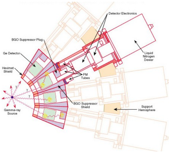
Fig. 4. Schematic of a modern escape-suppressed spectrometer array.
