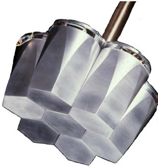
Fig. 18. The seven encapsulated Ge detectors of a Euroball cluster module.
