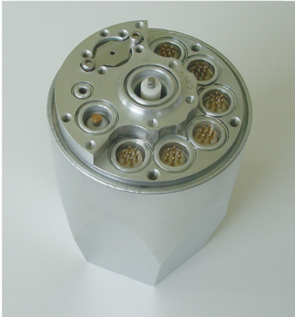
Fig. 31. The 36-fold segmented, encapsulated AGATA Ge detector.
