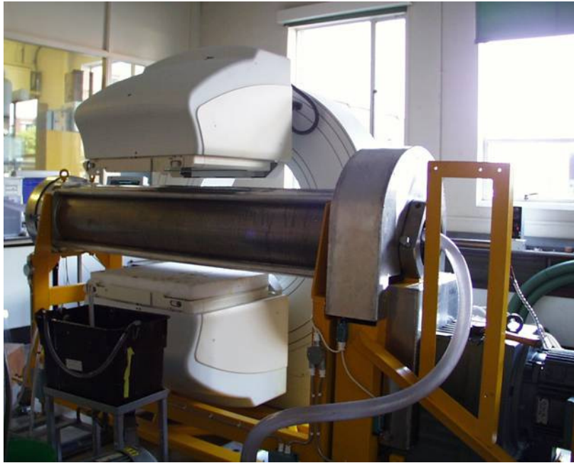
Scraped-surface heat exchanger
