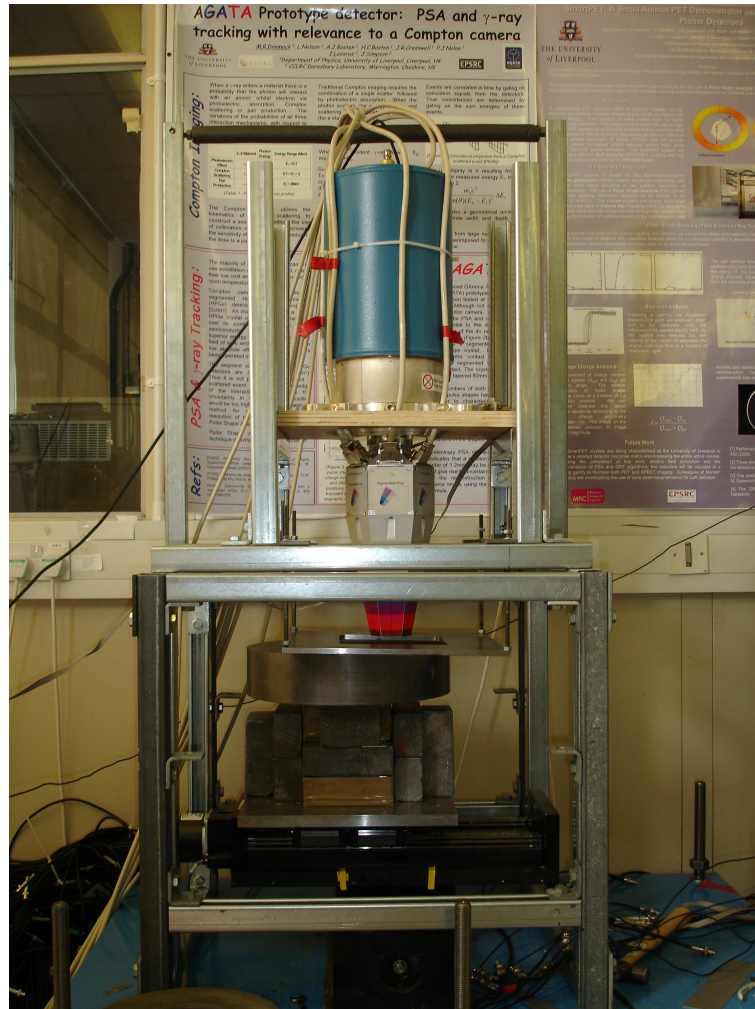
Figure 5.1: Photograph of the S002 AGATA prototype detector in position for the front face singles scan. The collimation system comprised of lead bricks and a lead collar can be seen sitting upon the scanning apparatus. The detector is suspended over the collimator by a wooden plate beneath its dewar so that the scanning table, source and collimation system are free to move beneath it.
