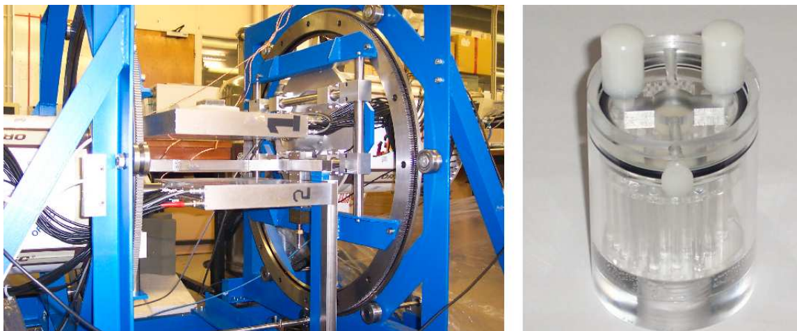
Figure 7.1: Left: SmartPET detectors housed within the supporting frame structure designed for the project. Right: Jaszczak cold rod micro deluxe phantom.
