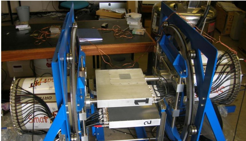
Figure 3.4: Both detectors sitting in their rotating gantry. The gantry permits PET and Compton camera studies and is controlled via 'in-house' MIDAS software. The gantry uses a holding torque to hold the detectors horizontal.
