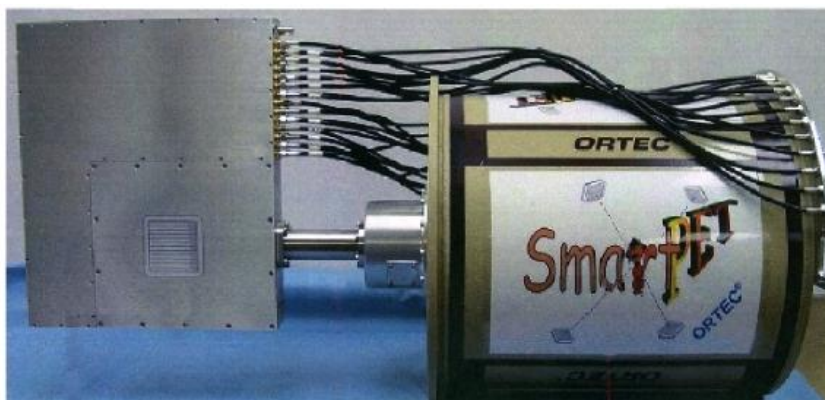
Figure 3.1: Photograph of SP1. The crystal is housed behind the small window in the cryostat which is marked with the electrode segmentation. The preamplifiers are read out from the black cables. The copper cold finger runs through the tube from the crystal to the dewar.
