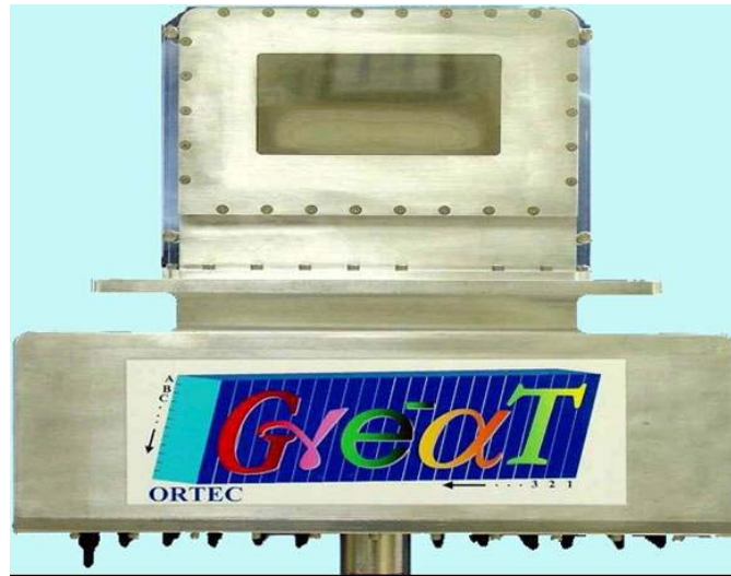
Figure 3.1: Photograph of the GREAT planar detector
