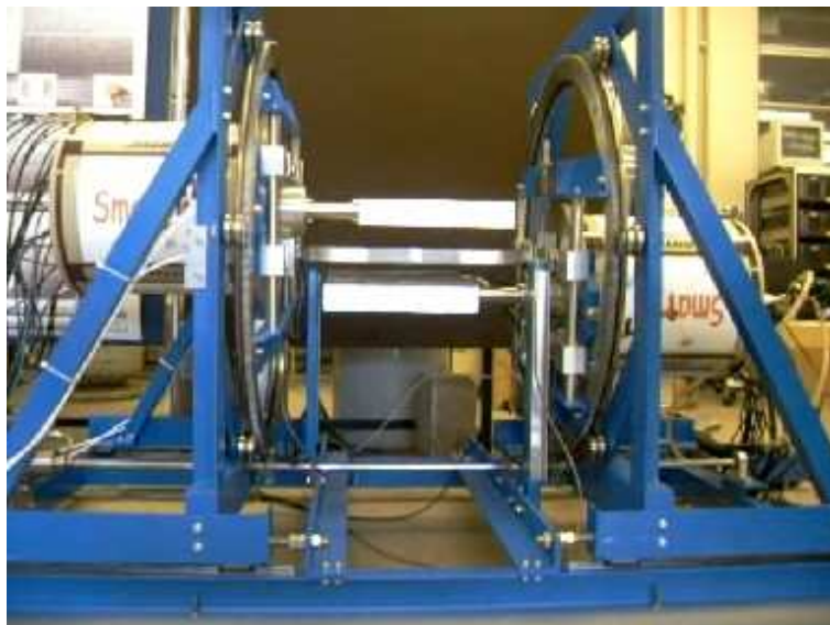
Figure 6.1: The SmartPET detectors in the automated rotating gantry for data acquisition in PET mode. The structure between the two SmartPET detectors at the centre of the field of view is the gantry sample tray designed to house the source to be imaged.
