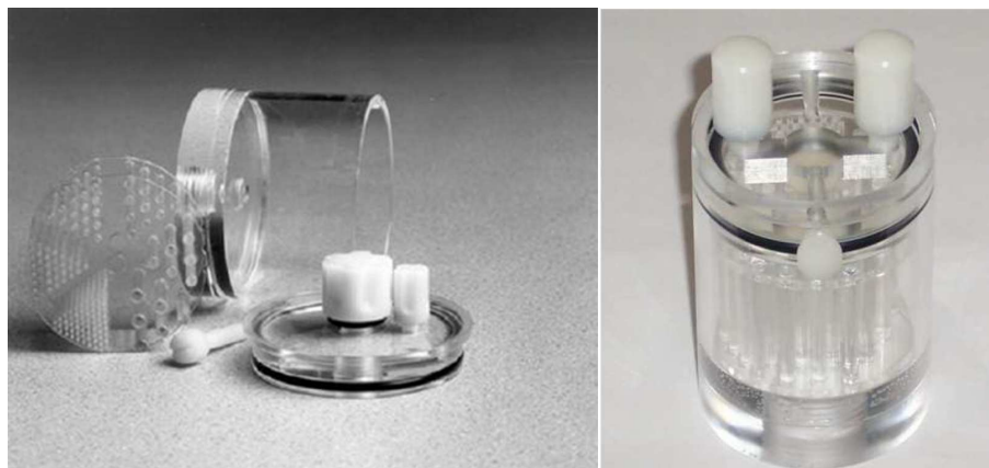
Figure 6.4: Pictures of a Micro Deluxe Flanged Jaszczak phantom. The image on the left shows the insert consisting of rods of various diameters.
