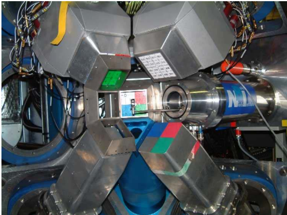
Figure I.1: picture of EXOGAM during the positioning of the detectors prior to an experiment. The two detectors at the top are EXOGAM Clovers equipped with the rear side elements of the escape suppression shield. The two small size detectors at the bottom are prototype segmented Clover detectors.
