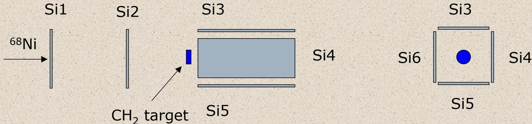
Target and detectors Si3 – Si6 are inside CsI ball
