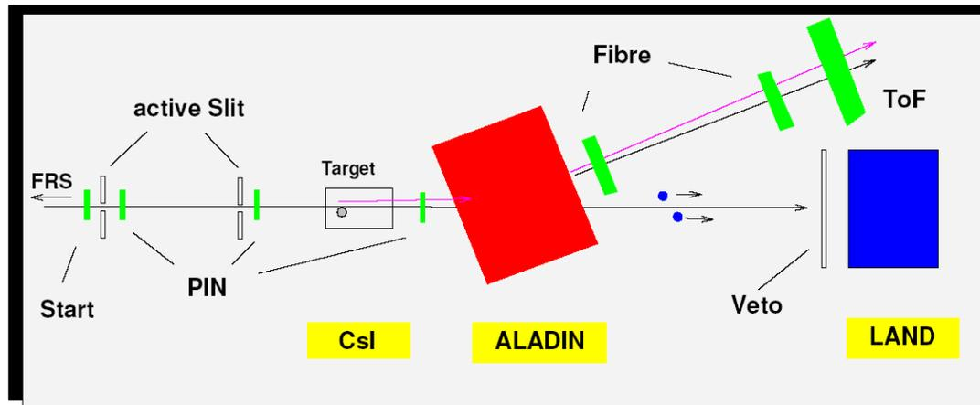
FIG. 3: Schematic view of the experimental setup (not on scale).
