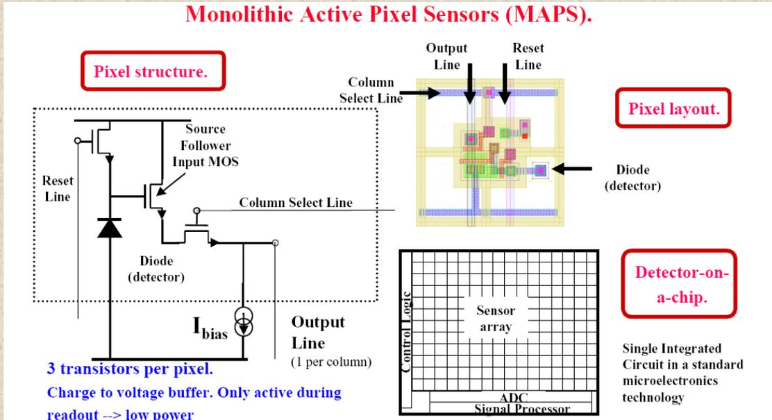
+ Detector and readout electronics on the same Si crystal
