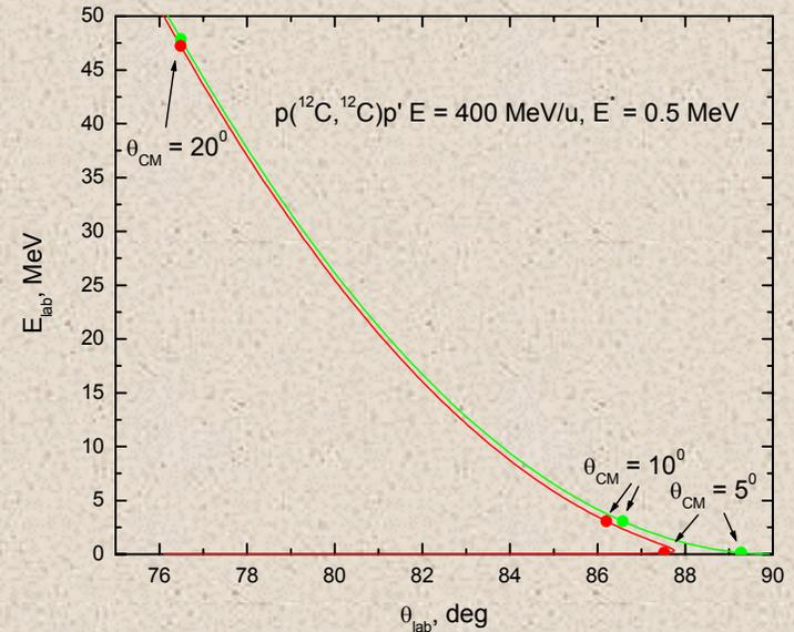
Recoil protons are coming out of the target, generated according to the cross section and the kinematics for elastic and inelastic scattering on  $^{12}\text{C}$
